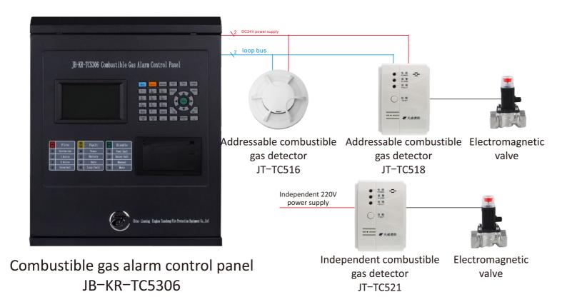
Combustible Gas Alarm Control System detects combustibility in industrial environment and daily living environment (such as kitchen using natural gas) When gas leaks and the combustible gas alarm control panel detects that the concentration of combustible gas reaches the alarm value set by the alarm, combustible gas alarm will send out sound and light alarm signals to remind people to evacuate, force exhaust and shut down the installation. Prepare for safety measures.
